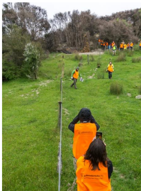
Fig. 19. 10 meter laterally offset fence on the Kekerengu fault rupture (photo credit: N. Wechsler).
